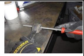
Clean the inside of the track bar tube on both ends with a file of sandpaper.
