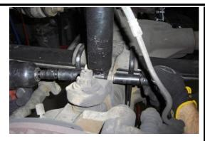
Support the front axle with a hydraulic jack. Starting on the driver side, unbolt the lower shock from the mount using a 21mm socket wrench.
