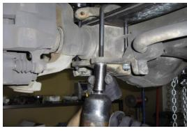
Remove the u-bolt nuts and u-bolts.
