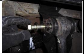
Install the .460 hex cam on the front side of the track bar bracket and the .390 hex cam on the back side. Install the 9/16-18x4" bolt, washers and nut.
