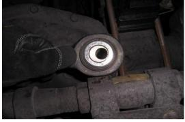
Rotate the sleeves so that the holes as far away from each other as possible.
