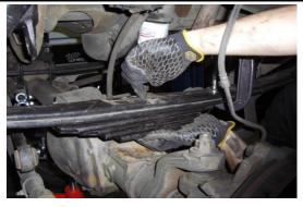
Install the ReadyLift mini leaf pack under the factory leaf pack using the new center pin bolt and nut provided. Tighten to 45 ft-lb.
