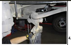
Rotate the axle mounting plate down out of the way.
