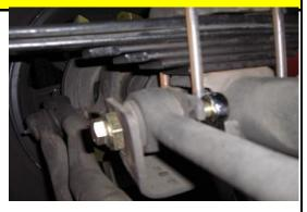
Install the .230 offset hex cams into the track bar bracket on the axle. Install the 9/16-18x3.5" bolt washers and nut. DO NOT TIGHTEN.
