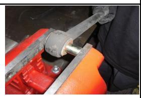
Press the offset drilled sleeves into the the track bar holes. DO NOT HAMMER!
