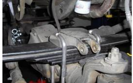
Install the upper mounting plate. Increasing the hole on the upper plate may be necessary in some cases. Install the u-
