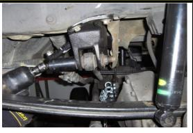
Remove the track bar using a 30mm socket or wrench at both the frame and axle.
