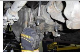
Rotate the axle pad up and install the u-bolt nuts and washers provided. Tighten to 125 ft-lb.
