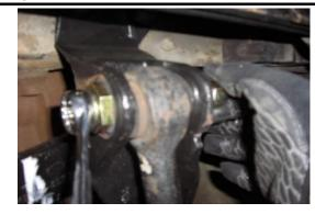
Tighten the track bar mounting bolts to 105 ft-lb.
