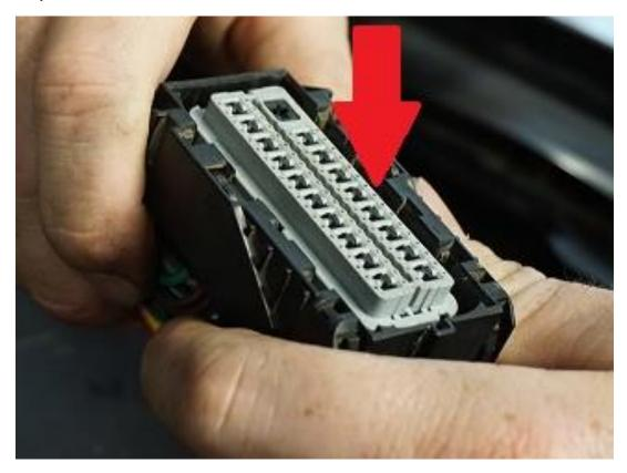
21. Using a zip tie fasten the wires to the plug where you use the snips to cut the original factory zip tie.
