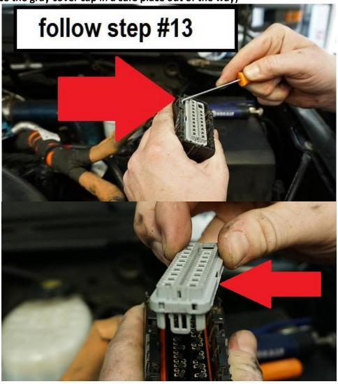
15. With the gray cap removed locate pin holes #11 & #35. 2011 model trucks will have a yellow wire running to pin #11. 2012 - 2016 model trucks have plastic filler pins in holes #11 and #35.
