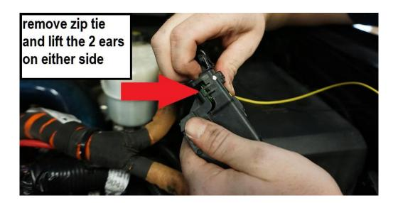
14. With the gray ECM connector in your hand use a pick/knife/flathead screwdriver to pry the gray cover off the bottom of the ECM connector. (Be very gentle as they can break very easy. Place the gray cover cap in a safe place out of the way)
