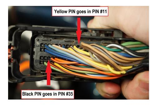
16. 2011 only - to remove the yellow pin from #11 use a small tool of some sort (paper clip) to put pressure on the release on the bottom side of the plug. (We used an angled pick to release pin #11)
