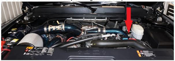
3. Remove the plastic protection cover by applying pressure to the tabs and sliding it out.
