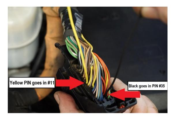
20. With both the Yellow and Black wires installed, put the gray bottom cover back on the plug. (make sure that it doesn't push the wires back out the top side when putting the gray cover back on)
