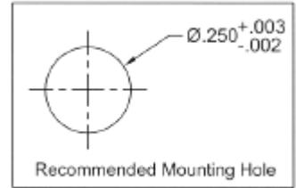
**IT IS CRITICAL THAT YOU CORRECTLY DRILL THE 1/4" PERFECTLY 90° OR PERPENDICULAR TO THE DRILLING SURFACE.**
