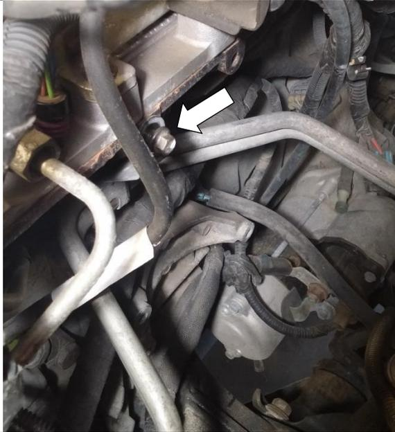
9. Remove the three (3) screws holding the bracket to the engine using a 10mm socket. Remove bracket from engine.
