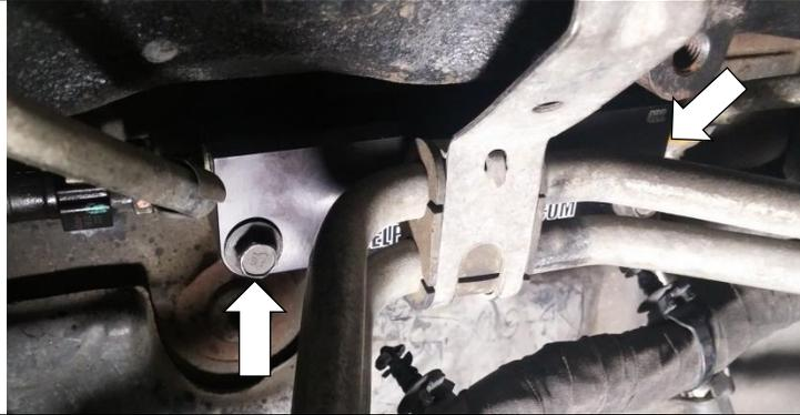
16. Slide a seal washer between the fuel block and return line, and install the original banjo bolt with the new washers. Do this on both sides.
