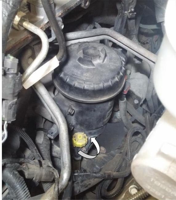
3. Disconnect the fuel heater and WIF sensor connectors.
