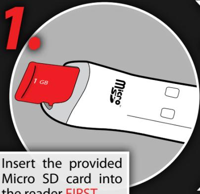
Insert the provided Micro SD card into the reader **FIRST**.
