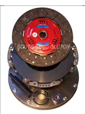
This clutch is designed for the moderately increased horsepower trucks 425 hp 900 torque. Offering a very smooth engagement with light petal effort. The perfect towing clutch.
