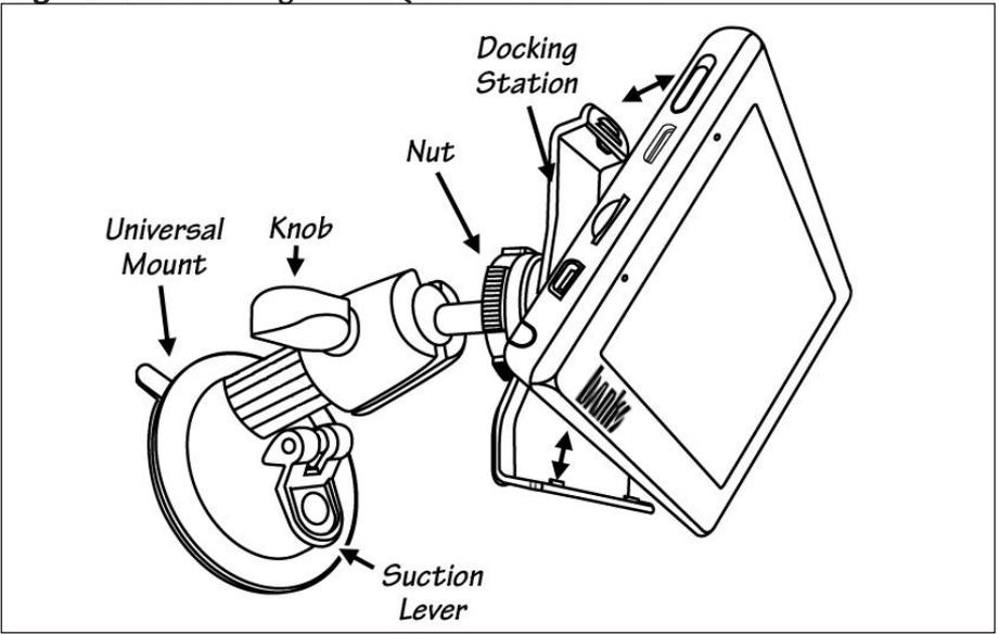
**5.** Make sure the suction cup and the mounting area on the windshield are clean and dry. With the suction lever in the up position, ensure the suction cup is flat against the windshield, and then push the suction lever down to secure in place.
