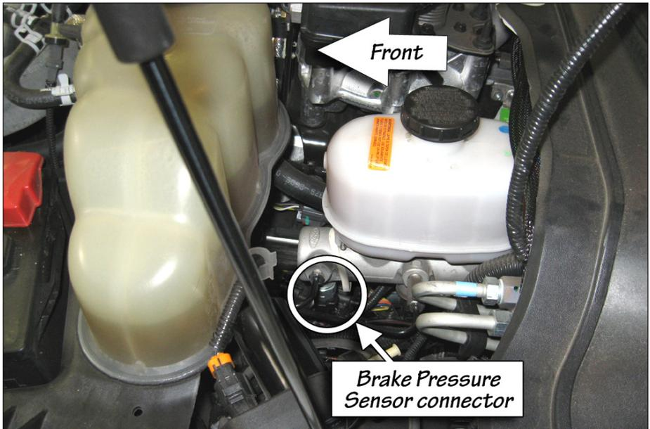
**6.** Locate the Banks Brake Wire Harness and connect the 2-pin male connector on the Brake Pressure Sensor harness to the 2-pin connector on the Banks Brake wire harness.
