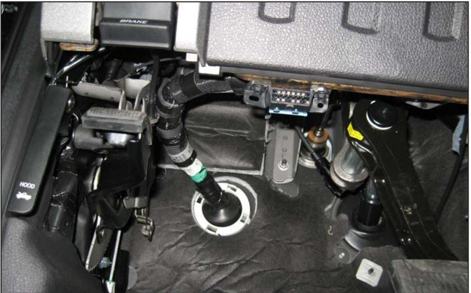
Now, feed the Six-Gun In-Cab cable on the Turbo/In-cab harness through the incision made in the firewall grommet and into the cab See **Figure 6**.
