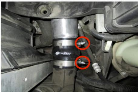
14. Place the other supplied T-bolt Clamp (I) over the end of the Straight Coupler (H).
