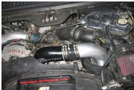
21. Reconnect both batteries. Inspect your installation, make sure the elbow and boost tube is properly positioned and all fasteners are secure. The installation is now complete.
