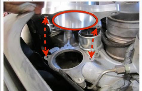
16. Install the other O-Ring (B) in the top groove of the Billet Spacer Block (A). Insert the S&B Intake Elbow (C) into the Straight Coupler (H) and align the mounting holes with the Billet spacer. Be sure both mating
