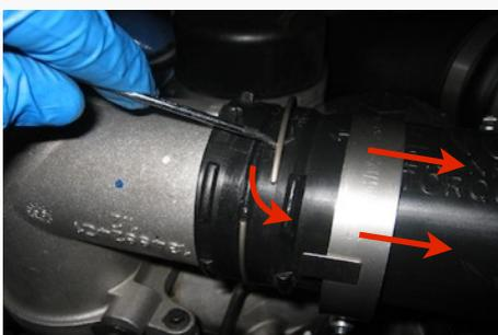
**5.** Loosen the hose clamp at the intercooler lower flange and remove the OE boost tube from the vehicle along with clamps. Remember how this is removed because it will have to be repeated to install the new one.
