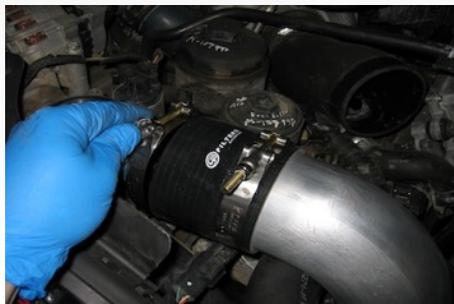
15. Clean the intake manifold surface. Then install the Billet Spacer Block (A) and the O-Ring (B) onto the intake manifold using 3 supplied M6x30mm Bolt (F) and 6mm Washer (D). Torque to 100 In.lbs.
