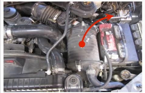
**4.** Loosen the upper hose clamp at the OE elbow and pry the compression clip out of the groove.
