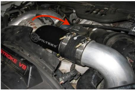
17. Insert the M6x30mm Bolt (F) and M6x93mm Bolt (E) in the proper locations and torque to 100 In.lbs.
