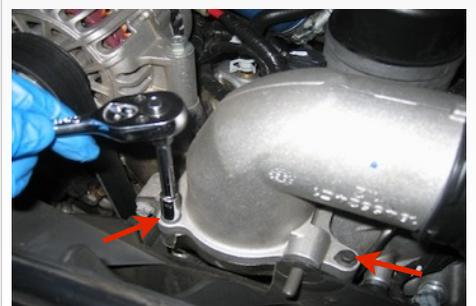
**7.** Apply sealant (Teflon tape) to each 1/8"NPT Plug (G) and insert the plugs into the ports you will not use on the elbow. Use 3/16" Hex drive and torque the plugs to 40 In.lbs.
