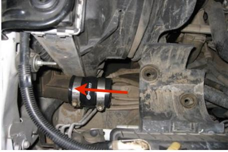
11. Place one of the supplied T-bolt Clamps (I) over the Straight Coupler (H) and slide it on the upper end (Large diameter) of the Boost Tube (J).
