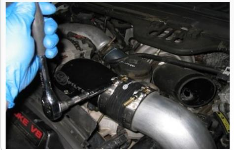
19. Reinstall the Intake or OE air cleaner and filter removed in Step 3.
