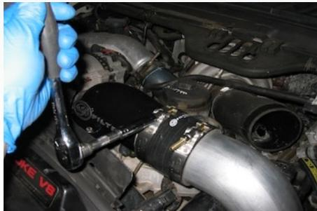
18. Reinstall the Intake or OE air cleaner and filter removed in Step 3.
