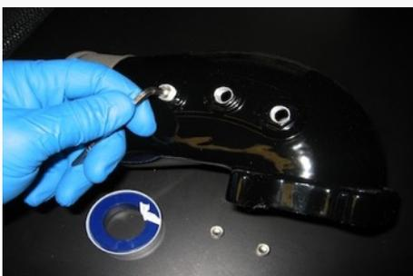
8. Place 6mm Washer (B) over each of the M6x30mm Bolt (D) and one over the M6x93mm Bolt (C), next apply a small amount of the supplied thread locker to each of the bolts.
