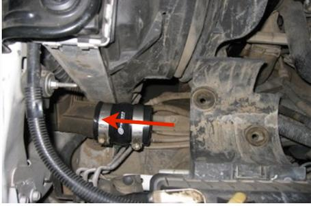
11. Place one of the supplied T-bolt Clamp (G) over the Straight Coupler (F) and slide it on the upper end (Large diameter) of the Boost Tube (H).
