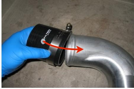
12. Snake the Boost tube assembly into position and into the Hump Coupler (I).
