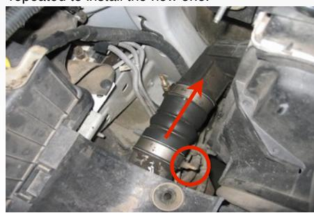
6. Remove the 4 bolts that secure the OE elbow to the intake manifold and remove the elbow from the vehicle. Be careful not to let debris fall into the intake manifold. *Note the longer bolt's location.*
