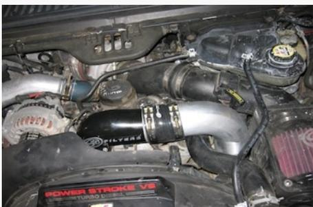
20. Reconnect both batteries. Inspect your installation, make sure the elbow and boost tube is properly positioned and all fasteners are secure. The installation is now complete.
