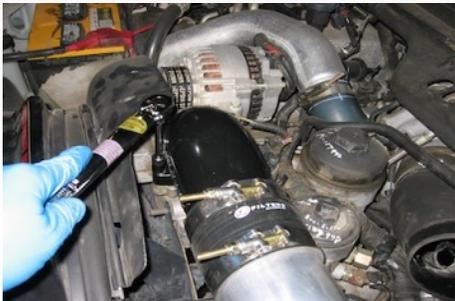
17. Position the upper T-bolt clamps as to not hit the hood when closed and torque them both to 50 In.lbs.
