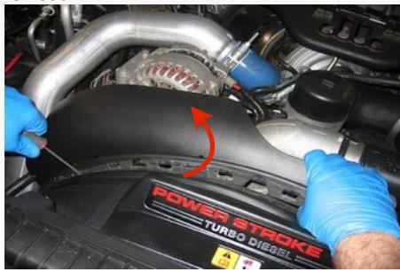
3. Remove the OE (or aftermarket) intake to gain access to the clamps of the OE boost tube. Follow the manufacture's procedures for removing the intake.
