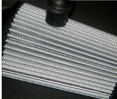
You can vacuum your Pro Dry S filter and return it to 96% of its original airflow. Remove the filter from the intake kit and vacuum away the dirt using a shop vacuum or regular house vacuum. Reinstall the filter in your vehicle. Do not apply oil to the filter.
