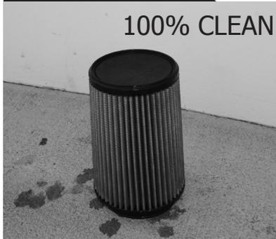
Allow the filter to dry completely (our synthetic media dries quickly and should dry within a few hours in normal conditions). Reinstall the filter in your vehicle. Do not apply oil to the filter.
