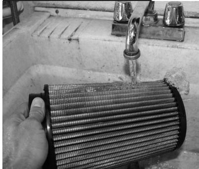
Rinse the filter with clean water to remove the dirt and excess cleaner. Continue rinsing until the water runs clear.
