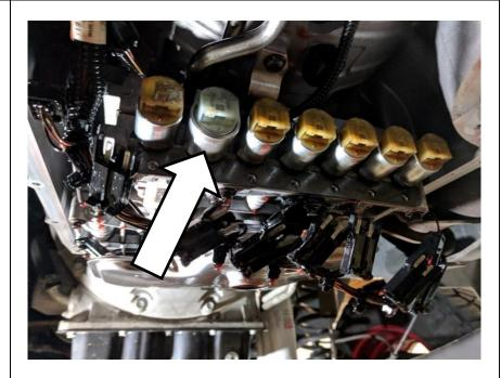
7. Secure the retaining plate and install connectors into solenoids.
