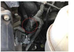
STEP 3 PLUG IN THE GDP 3 PIN UNLOCK CABLE
