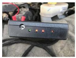
FLASH CODES: FLASH CODES ARE FLASHING LIGHTS ON EACH OF THE LED'S, THE NUMBER OF EACH ONE (RUNNING FROM LEFT TO RIGHT) WILL INDICATE THE ERROR EXPERIENCED.
