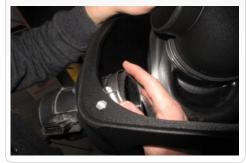
27. Install both Mounting Brackets (K) with grommets inside the vehicle on the plastic
