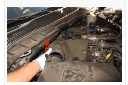
6. Use a 5/16" nut driver to loosen the hose clamp on the turbo inlet.
