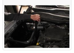
**31.** Install the S&B tube assembly and connect to the factory turbo inlet and tighten the hose clamp.
