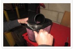
$26. \ \ \text{Install the Hose Clamp (H) onto the MAF} \\ \ \ \ \text{Adapter (B)}.$
