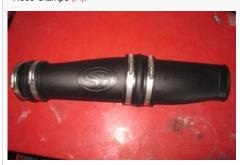
24. Install the Filter Adapter (G) onto the S&B Air Filter (J). Use a screw driver to lineup the S&B logo on the filter straight with the (-) on the part number of the Adapter
