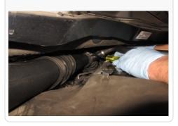
**32.** Slide the coupler towards the S&B air box over the MAF. Tighten down the hose clamp and make sure the tube is aligned properly.
