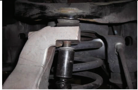
Loosen upper ball joint nut and break loose with hammer.
