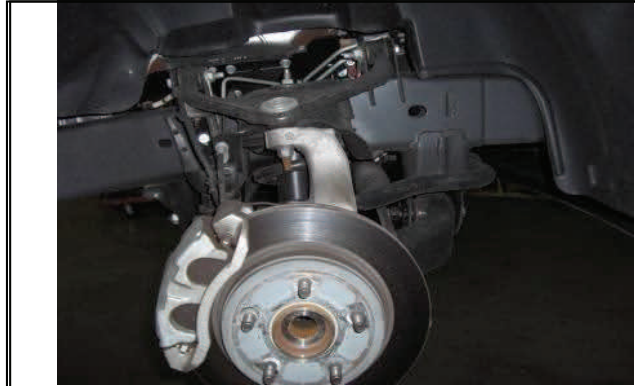
Remove front wheels and tires
