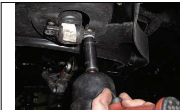
Disconnect lower shock mounting bolts.
