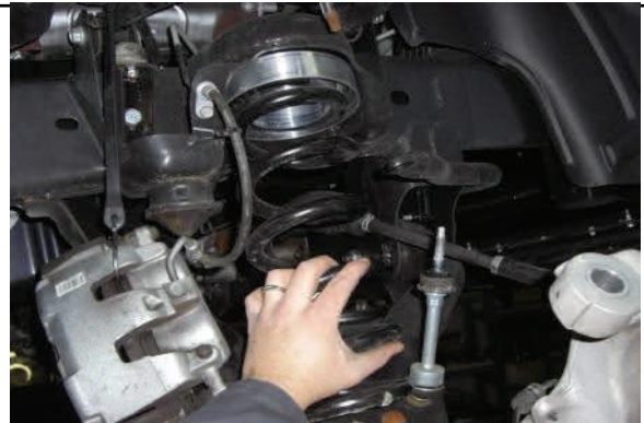
Reinstall coil spring and properly clock in lower control arm.
