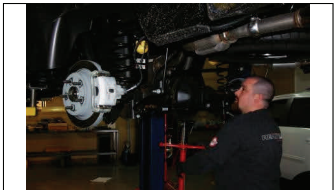
Reattach shocks, trac bar, sway bar end links, and ABS lines
