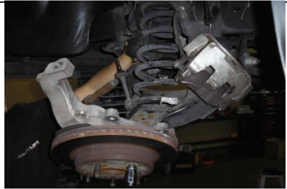
Slowly lower suspension and remove coil spring.
