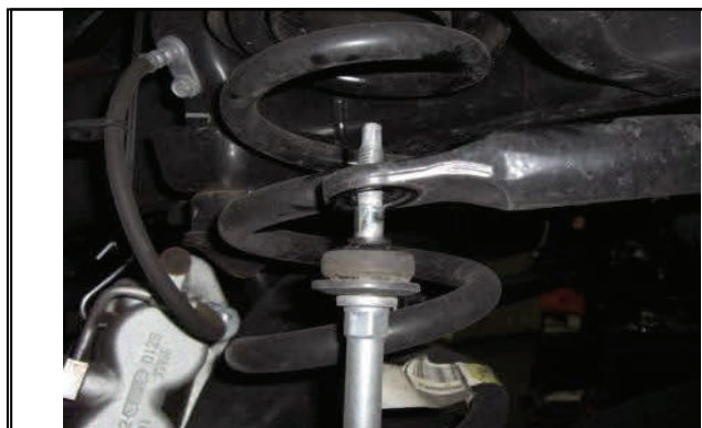
Disconnect upper sway bar end links and bushings
