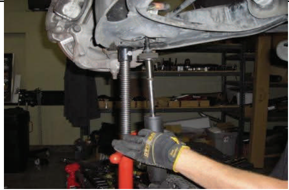
Reuse OE bushings and hardware top and bottom.
