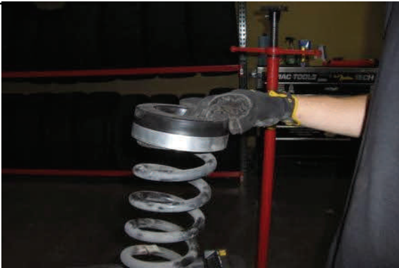
Remove upper isolator and replace with new ReadyLIFT hat.
