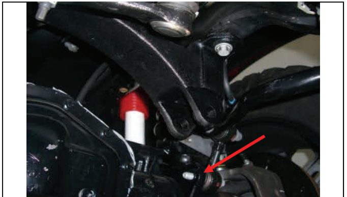
(05-10) Re-attach and tighten sway bar end links.
