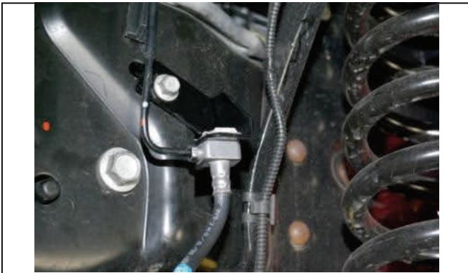
Reinstall block into bracket with retaining clip.
