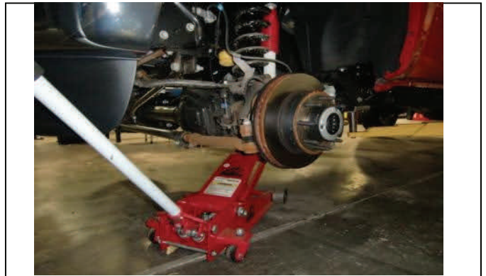
Support front axle with floor jack(s).
