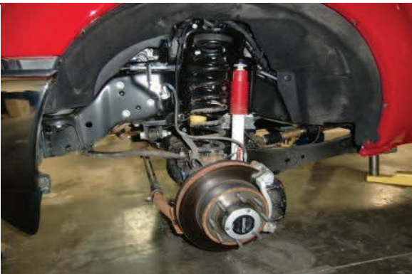
Remove front wheels and tires.
