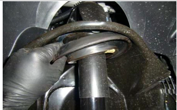
Remove Spring isolator if it did not come out with Coil Spring
