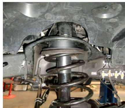
Re install Isolator and coil spring
