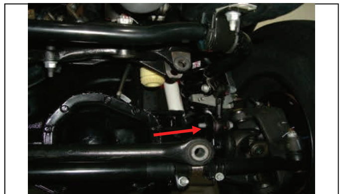
(05-10) disconnect dr/pass lower front sway bar endlink bolt.
