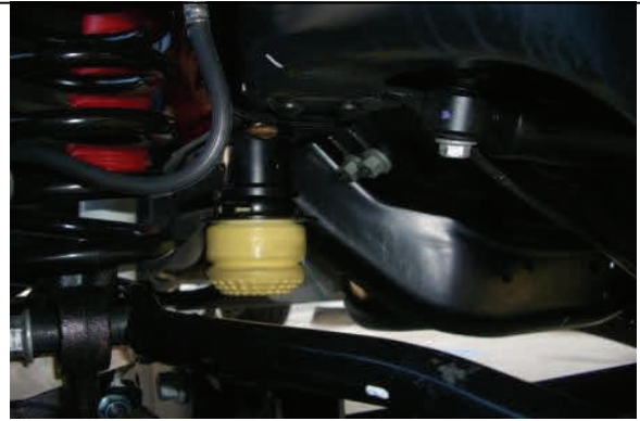
Assemble bump stop bracket to extension and reinstall.
