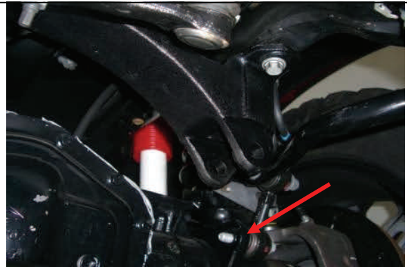
(.05-10) Re-attach and tighten sway bar end links.
