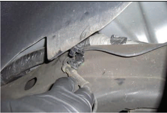
Follow line up and unclip ABS lines at frame
