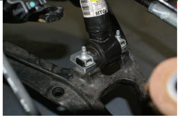
Install lower strut spacer and tighten,
