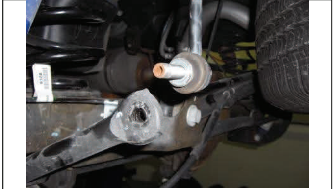
Support axle with jack and disconnect sway bar end links
