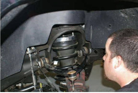
Place spacer on strut top and reinstall loosely with new nuts
