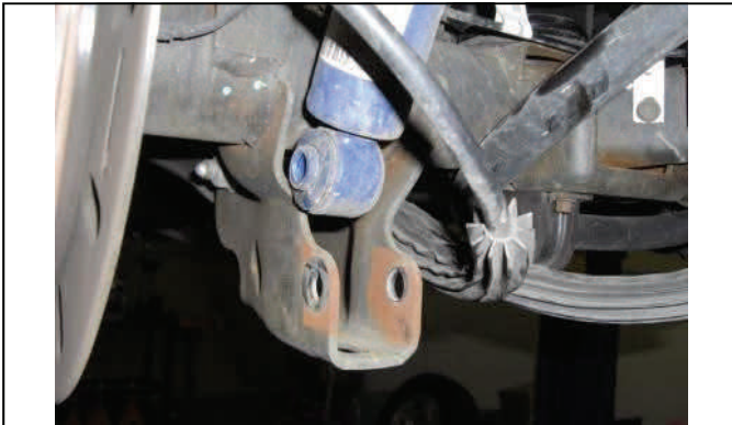
Disconnect Lower shock mounts
