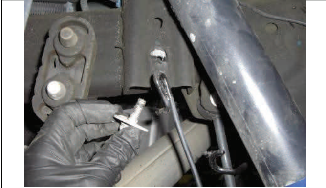
On the driver side frame unbolt e-brake hanger
