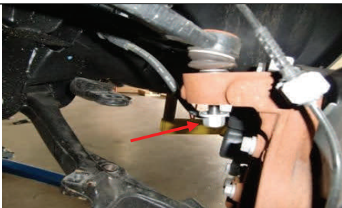
Support suspension loosen upper ball joint nut
