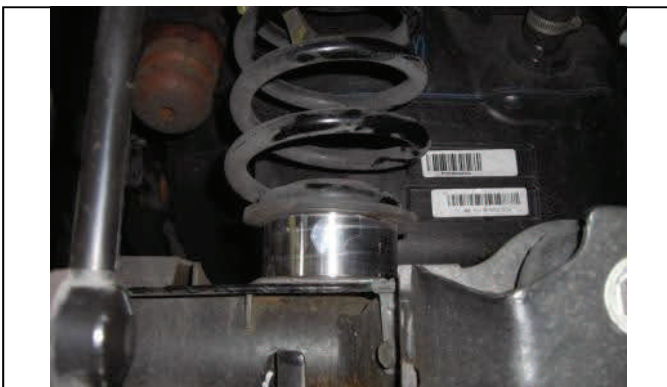
Reinstall coil spring and seat on top of spacer, raise axle.
