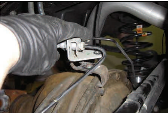
Disconnect brake lines at top of differential
