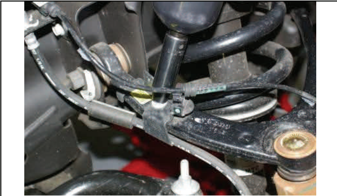
Disconnect ABS/brake bracket from upper control arm.
