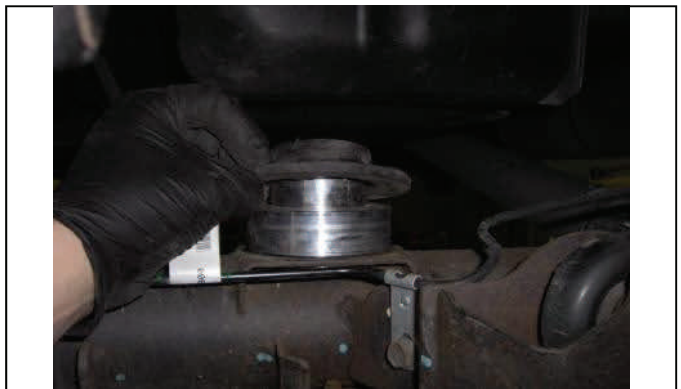
Refit OE rubber isolator on top of billet spacer
