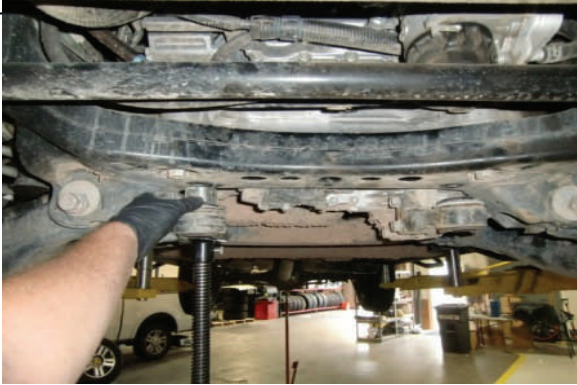
4WD Slowly lower to allow spacers to be placed as shown.
