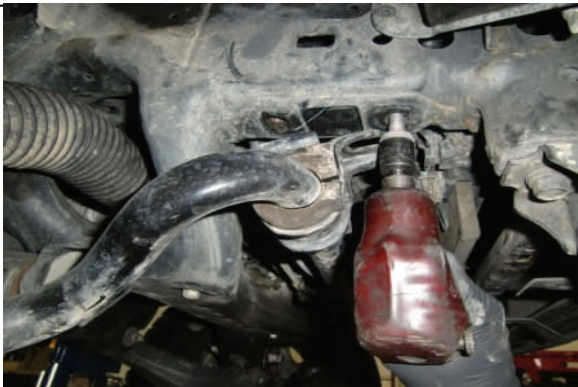
Disconnect sway bar at the frame mounts.
