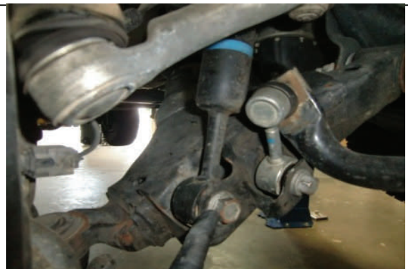
Position lower strut mount into position, use OE hardware.
