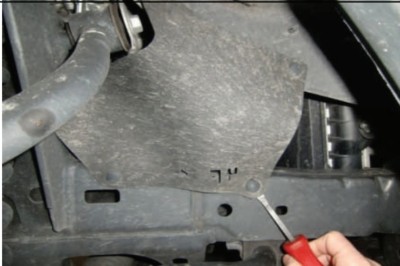
Remove splash guards at frame in front of upper control arms
