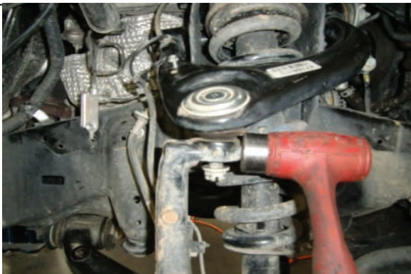
Separate upper ball joint from upper control arm.
