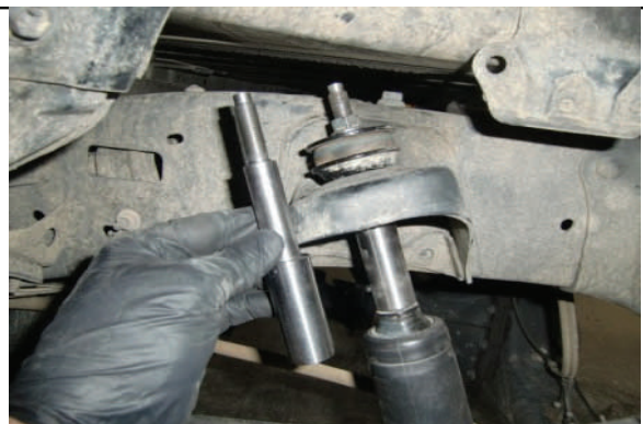
Install provided upper shock extension as shown.
