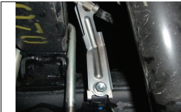
Remove brake line bracket bolt from axle tab.
