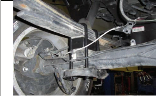
Attach lower mounting plate with provided hardware.
