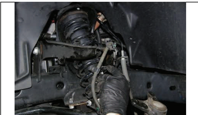
Remove upper strut mounting hardware. Remove strut
