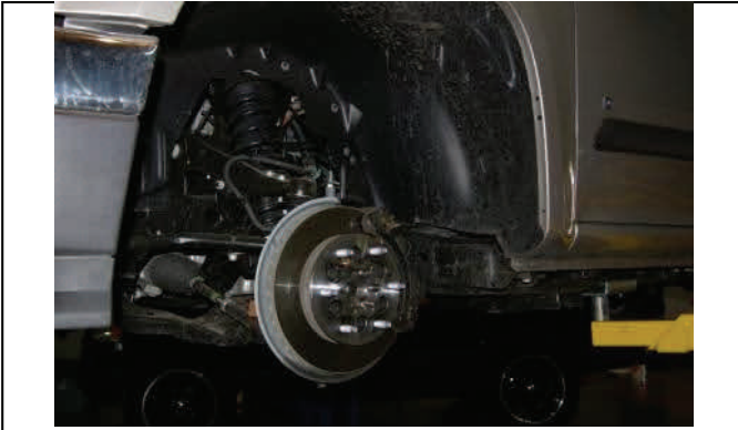
Raise and support vehicle frame and remove wheels/tires
