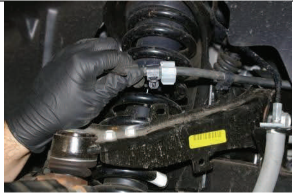
Unclip brake lines from upper control arms
