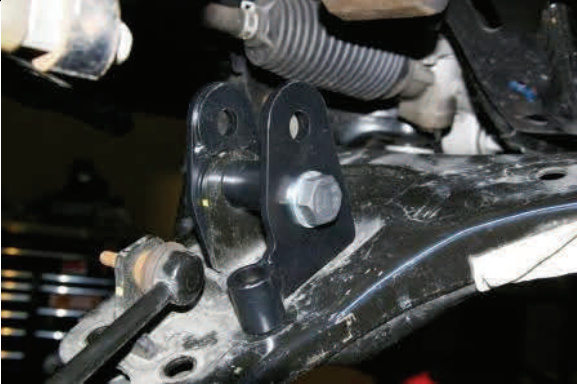
Assemble lower strut extension brackets as shown
