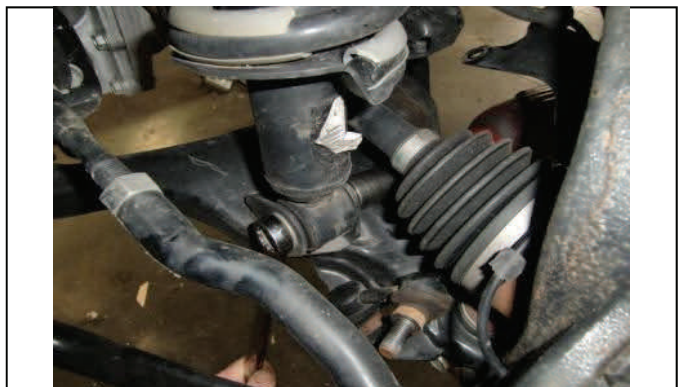
Remove lower shock mounting hardware
