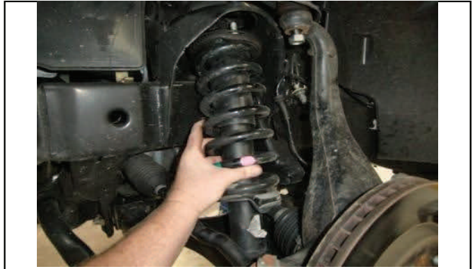
Remove strut assembly from vehicle
