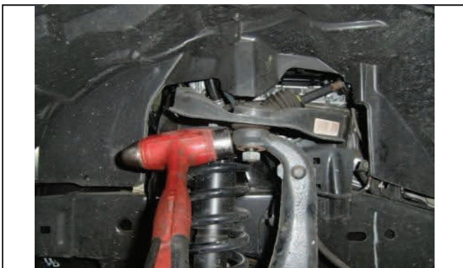
Strike spindle to break loose connection
