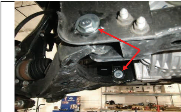
Orient cams in the upright/neutral position and tighten
