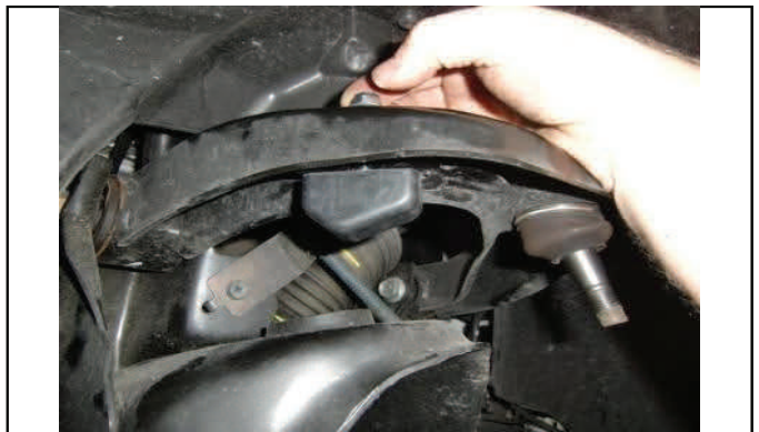
Attach bump stop as shown, note bumpstop orientation
