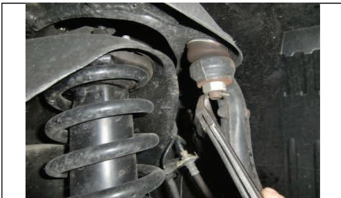
Remove cotter pin and upper ball joint
