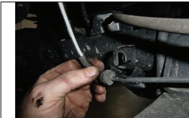
Remove ABS lines from attachments on axle
