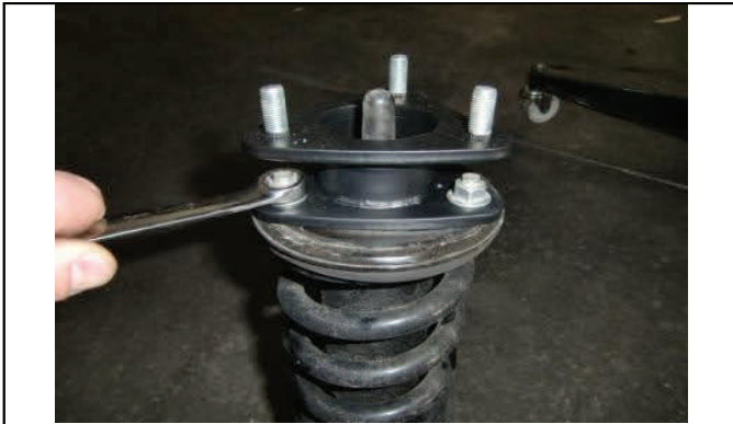
Attach strut extension with OE hardware
