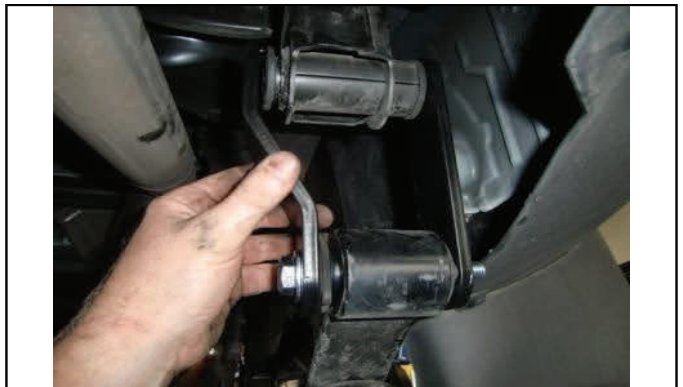
Attach new inner brackets and hardware
