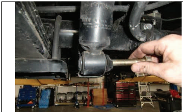
Remove lower shock mounting hardware
