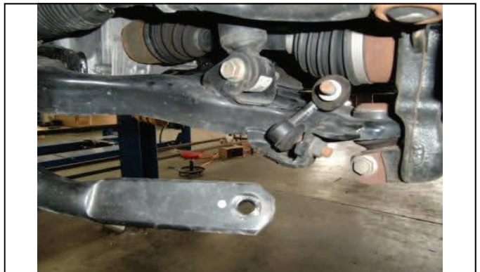
Disconnect sway bar end links
