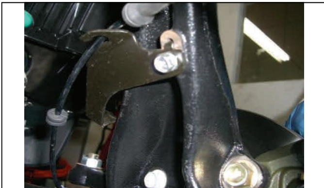
Disconnect ABS line bracket behind spindle
