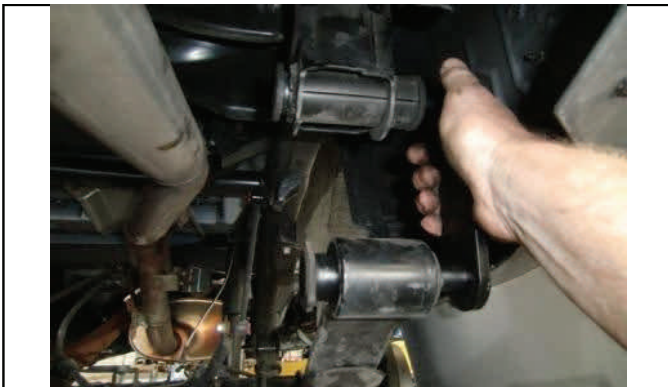
Lower axle and install new shackle bracket
