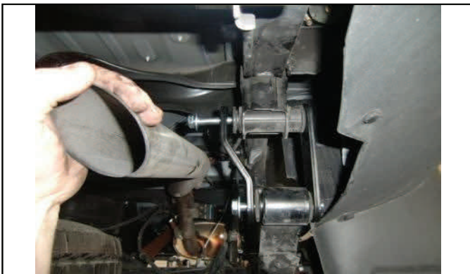
On passenger side, pull down on exhaust to gain access
