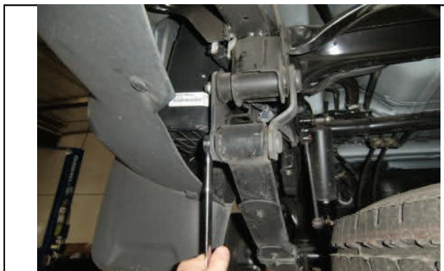
Unbolt the upper/lower shackle hardware
