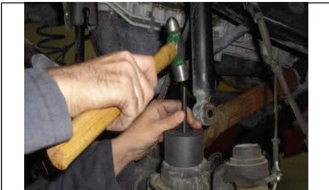
Center, mark and drill 11/32 hole for self tapping bolt.
