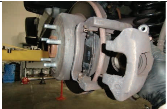
Remove rear brake calipers.
