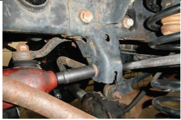
Support front axle and remove upper trac bar bolt.
