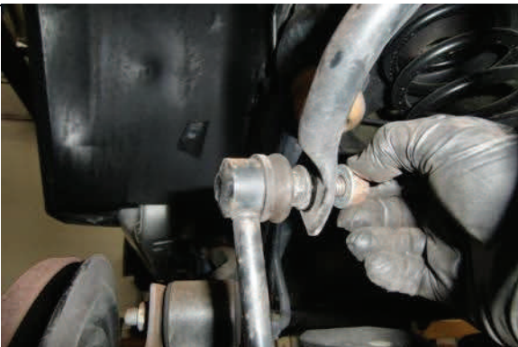
Disconnect rear sway bar end links
