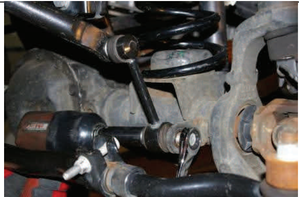
Disconnect dr./pass. lower front swaybar endlinks
