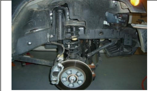
Carefully raise vehicle off ground and remove (4) wheels
