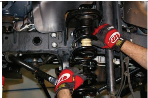
Carefully lower front axle remove springs and rubber isolator.
