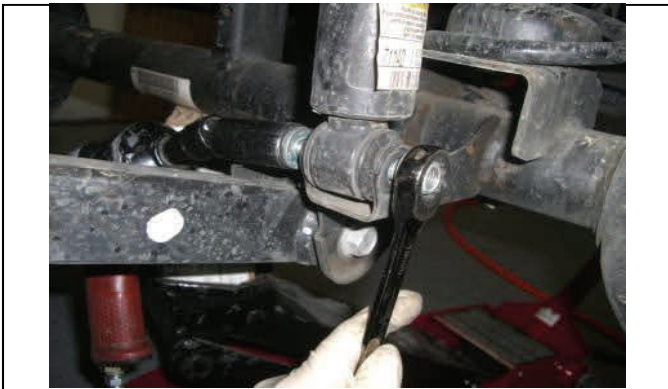
Disconnect and remove front lower shock hardware.
