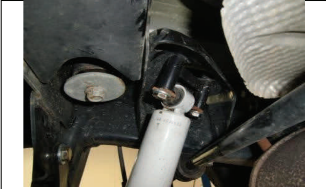
Install upper shock extensions with provided hardware.
