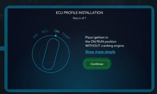
Place the ignition in the ON/RUN position WITHOUT cranking the engine.
