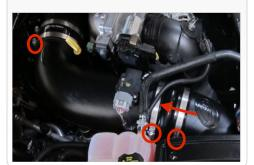
24. Reconnect the MAF sensor wiring harness. Reconnect the Humidity sensor wiring harness if applicable.
