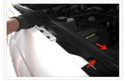
6. For 2015-2016 Models Only. Remove both the upper and lower crossbars by removing the 5 mounting bolts, a 10mm & 13mm socket will be needed. The lower crossbar bolt can be accessed by pulling up on the front plastic liner.
