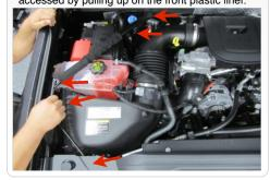
7. Loosen the hose clamp connecting the intake tube to the air box lid. Then remove the intake tube from the truck.
