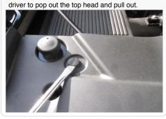
5. For 2015-2016 Models Only. Remove the rubber hood seal on the passenger side by pulling forward towards the front of the hood and pulling up.
