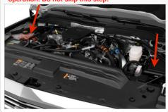
2. Disconnect the electrical connection for the MAF sensor. For 2013-2016 Models, disconnect the electrical connection for the humidity sensor.
