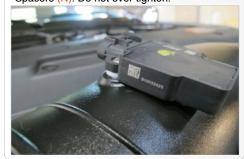
13. For 2011-2012 Models Only. Install the Block Off Plate and Gasket (S & T) onto the Intake Tube #2 (K) with the M4 Screws (O).
