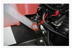
12. Carefully remove the MAF sensor from the stock air box lid and install the MAF sensor onto the Intake Tube #2 (K) with the supplied #8-32 Screws (R) and Plastic Spacers (N). Do not over tighten.
