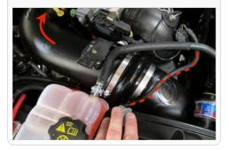
23. Make any adjustments to the tube if necessary, when satisfied with the positioning, tighten all hose clamps. Do not over tighten.
