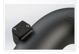
14. For 2013-2016 Models Only. Carefully remove the humidity sensor from the stock air box lid and install the humidity sensor onto Intake Tube #2 (K) with the supplied M4 Screws (O). Do not over tighten.
