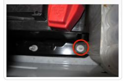
11. Unsnap the plastic clip holding the coolant reservoir to the AC line using a flat blade screwdriver. Then remove the other screw mounting coolant reservoir.
