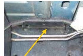
**NOTE:** Some pickup model frame rails have a bracket that is used to support the frame during the manufacturing process. If this bracket is on your frame rail and obstructs the proper positioning of the Raptor™ mounting bracket, you may remove it! Be very careful not to damage the frame.
