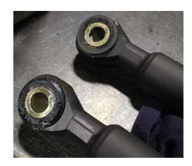
Thread one ¾"-16 nut onto each rod end (1302133) and install into rod.
