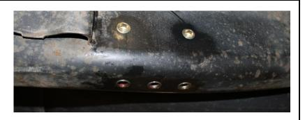
11. Mount both frame mount brackets to the frame using the 3/8"-16 serrated flange bolts. Use blue thread lock on all bolts and torque to 30 ft-lbs.
