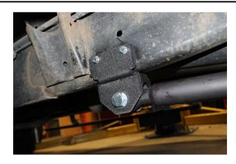
Use the 1/2" washers and 13. tighten the 1/2"-13 U-bolts in a cross pattern to 95 ft-lbs. Ensure the U-bolts are square to the axle when installed.
