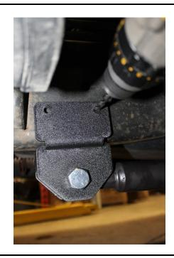
6. Gradually increase the drill bit size until the hole is 17/32" (0.531") in diameter. Deburr or smooth the leading edge of the drilled hole and apply a small amount of paint to resist corrosion.
