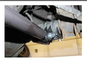
14. Torque the 3/4"-16 jam nuts to 145 ft-lbs. Use a flat head screwdriver to centre the rod end during torqueing.
