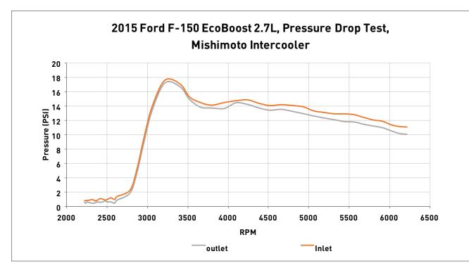
FIGURE 5: Mishimoto Intercooler pressure drop across the intercooler during a dyno pull. At the end of the run there is about a 1 psi pressure drop.
