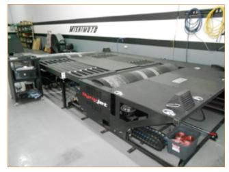
FIGURE 3: A Dynojet<sup>TM</sup> dynamometer was used for vehicle testing.
