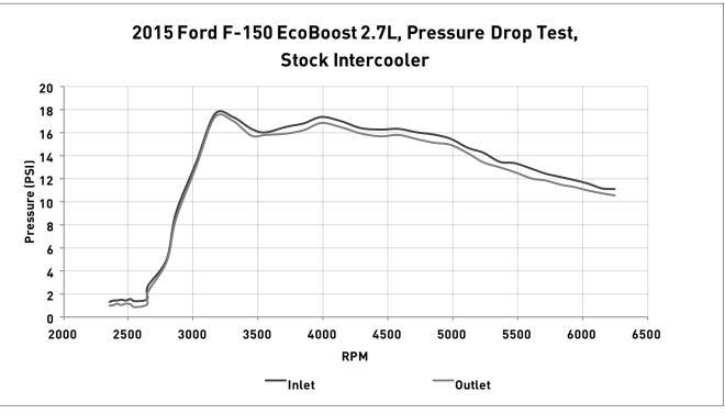
FIGURE 6: Stock intercooler pressure drop across core. At the end of the run there is about .75 psi.
