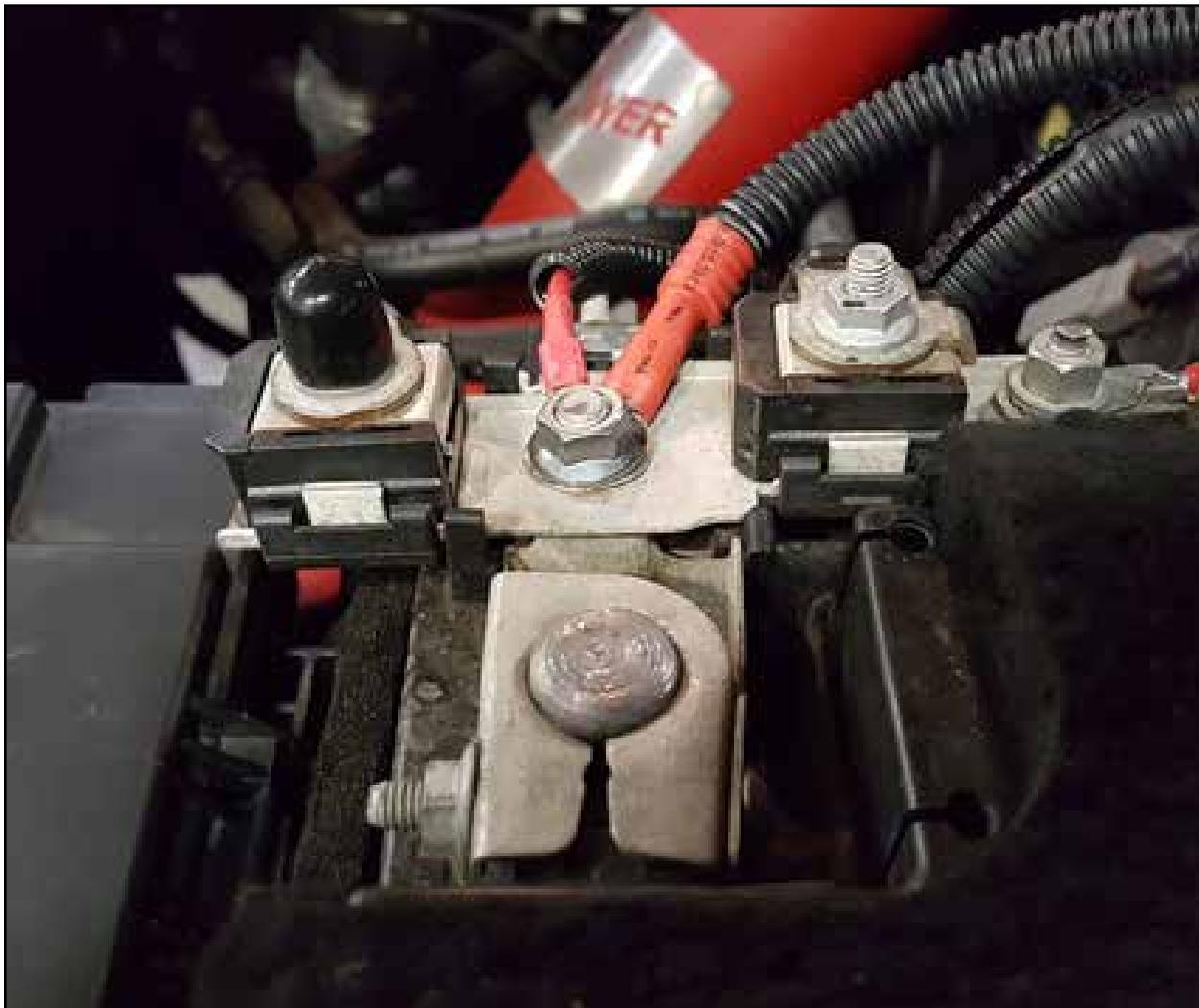
Step 29: Connect the red wire ring terminal on the power harness to the positive side of the battery.
