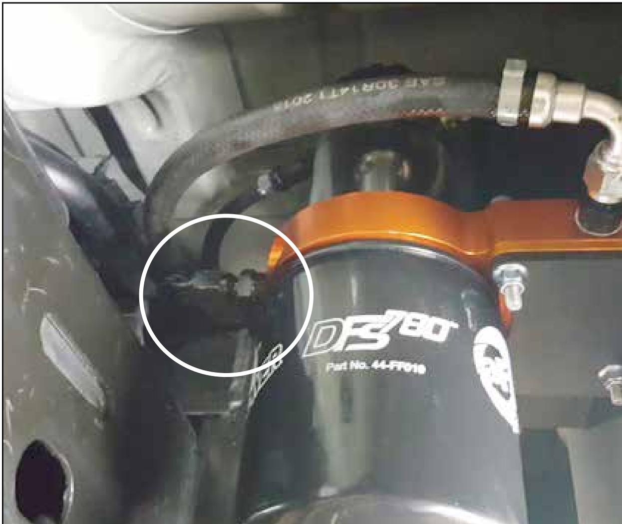
Step 19: Install the fuel outlet hose (black 90° -6 AN fitting) onto the male -6 AN fitting on the fuel outlet port of the fuel manifold assembly and tighten.
