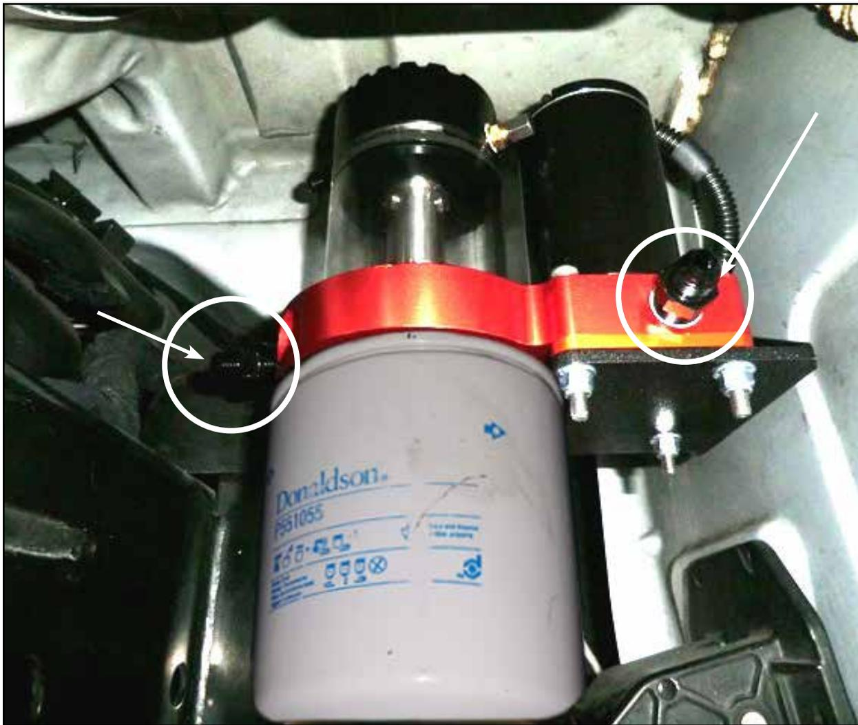
Step 8: Install the 2 x 3/8" NPT to -6 AN fittings into the fuel manifold assembly (as shown above).
