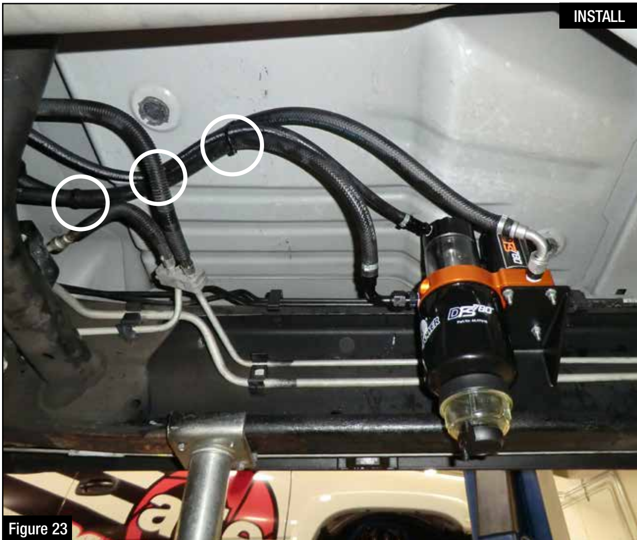
Step 24: Using the supplied nylon cable ties, secure the new hoses (as shown above).
