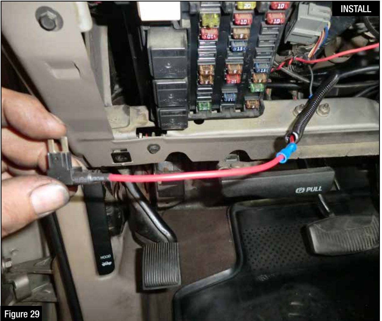
Step 33: Attach the power wire from the relay to the inline fuse adapter.
