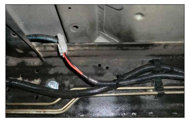
Step 16: Plug the Deutsch connector on the end of the supplied power harness into the mating connector on the fuel pump motor.
