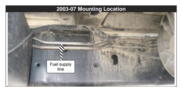
4. Cut the steel fuel supply line and remove a 14" section, centered on the location you chose to mount the mounting at. A pipe cutter is strongly recommended to cut the line, be sure not to squish or compress the fuel line, and remove any burrs that are left over from the process.
