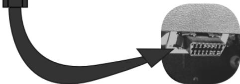
**STEP 1** - Plug the device into the OBDII port.
