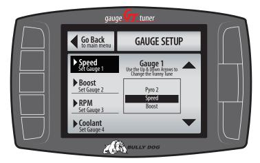
3. Use the buttons on the right side of the GT Platinum to scroll through the different functions and highlight the one you want shown on the General Display.
