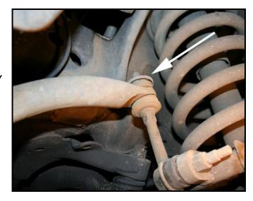
Apply Loctite and install (snug, not tight) four of the supplied 17mm bolts with washers to re-secure the sway bar and SBS to the frame, while allowing the final mounting position to be fine tuned.
