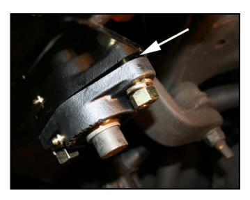
Tighten the four sway bar mounting bolts (17mm) to 40 lbs-ft. (as per Dodge's specification).
