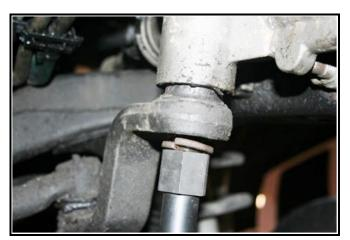
Slide the SBS bar into place, where the mounting feet are positioned in between the sway bar mounting and the frame.
