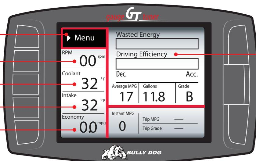
**Vehicle parameters:** To change which vehicle parameter is displayed in the large gauge area, simply press one of the four buttons next the preferred vehicle parameter.
