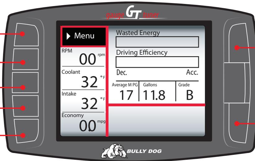
**FUNCTION 2:** Press any of the four buttons on the left side of the GT Platinum adjacent to one of the vehicle parameters on the screen will display that parameter in the large gauge area.
