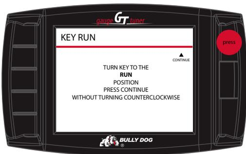
Check battery and connect charger if needed. If output is  $\leq 12V$ , installation will not continue until at least 12.1V is available.
