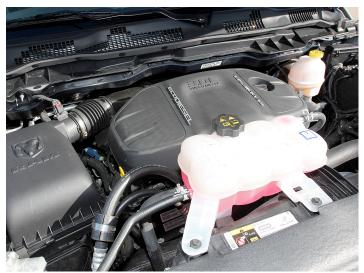
**3.** Remove the air filter tube and the foam padding under the engine cover.
