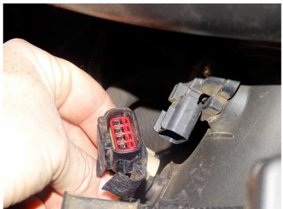
5. Now route the EcoPro wire harness back to the MAP sensor, identified in this picture with the red circle. Disconnect it and connect the middle set of connectors on our harness to both the sensor and the factory harness.
