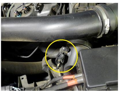
4. Disconnect the factory harness and connect the set of connectors at the end of our wire harness. You will connect our harness to the sensor and to the factory wire harness.
