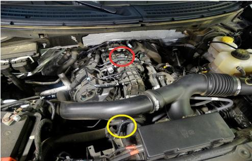
2. Now you will want to locate the Turbo Charger Pressure Sensor and the MAP Sensor both shown on this picture. The Turbo Charger Pressure sensor is identified with the yellow circle while the MAP sensor is identified with the red circle.
