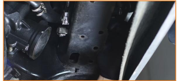
2. Remove the bolts where the frame ends meet the bumper. (2x 18mm bolts)
