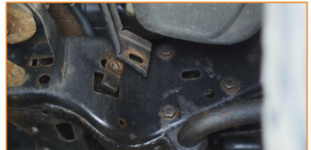
3. Remove the bolts and brackets that secure the front bumper. (6x 18mm bolts)
