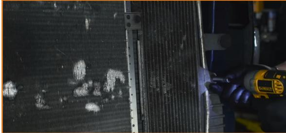
7. Install the Mishimoto transmission cooler. (2x10mm nuts, 1x 10mm bolt)
