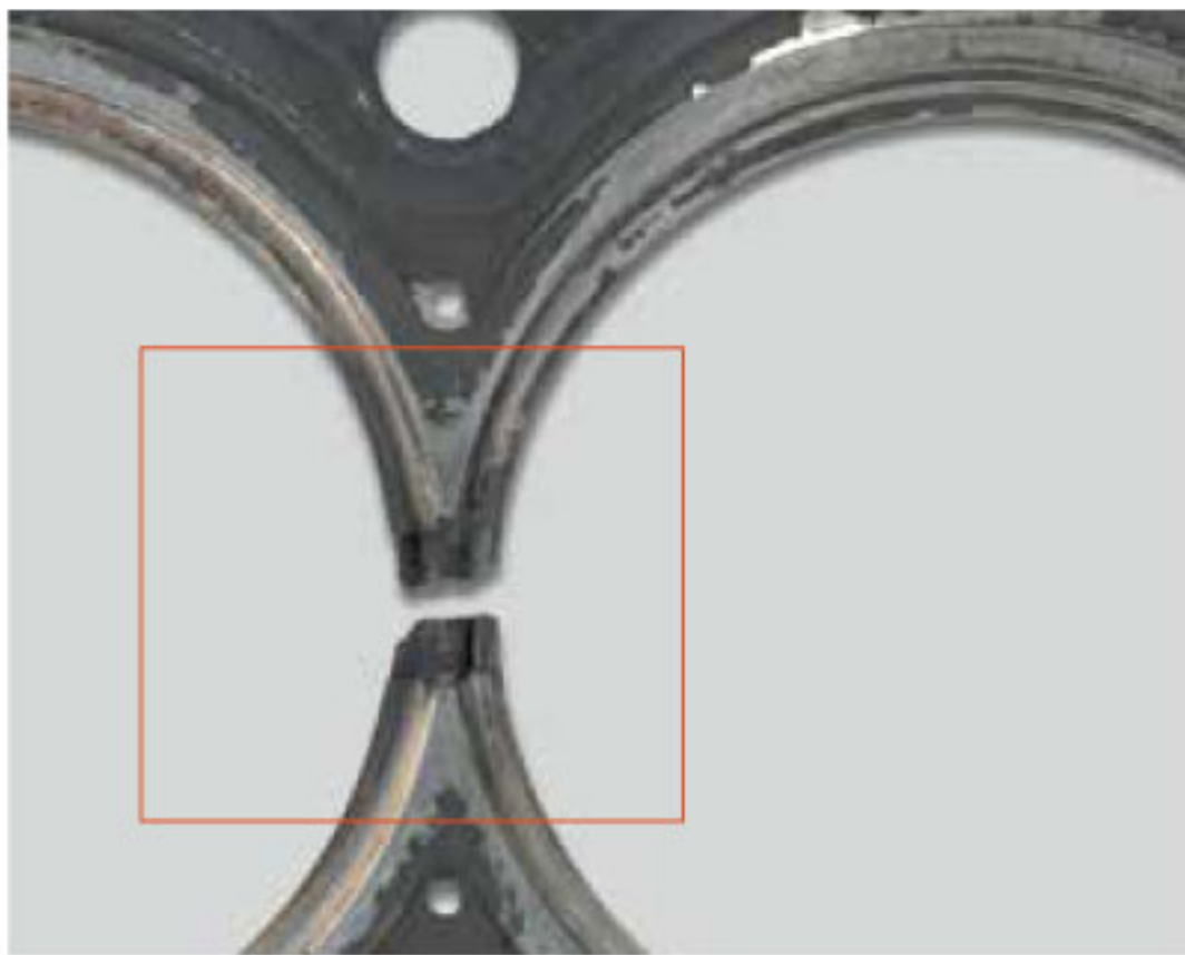
▲ Broken web caused by high component dynamics
