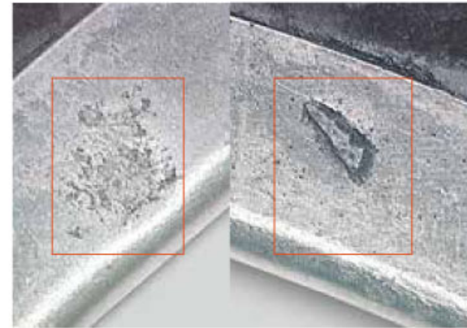
▲ Gasket damage due to dirt and foreign objects.
