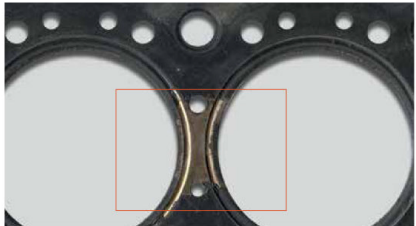
▲ Scorched elastomer coating
