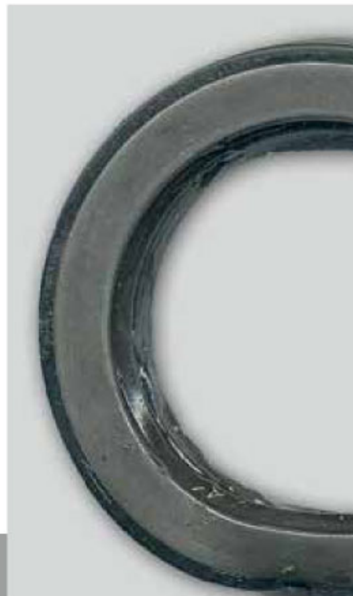
▲ Greased PTFE sealing lip as the cause of failure.
