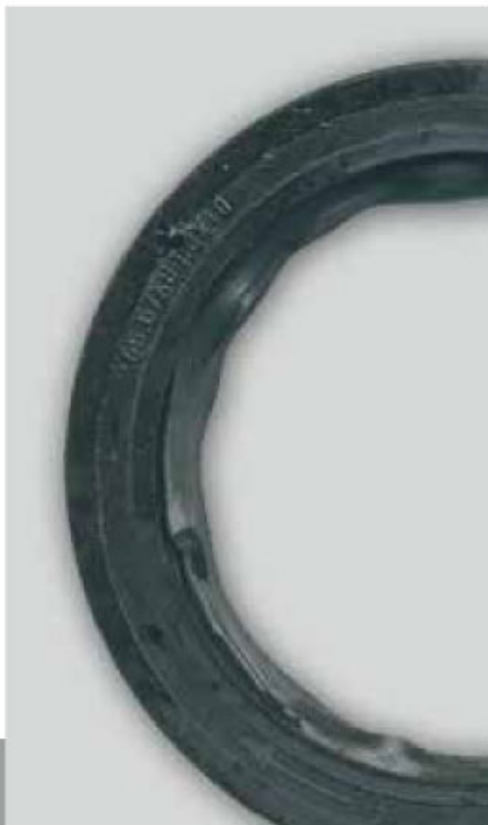
▲ Damaged PTFE sealing lip as the cause of failure.
