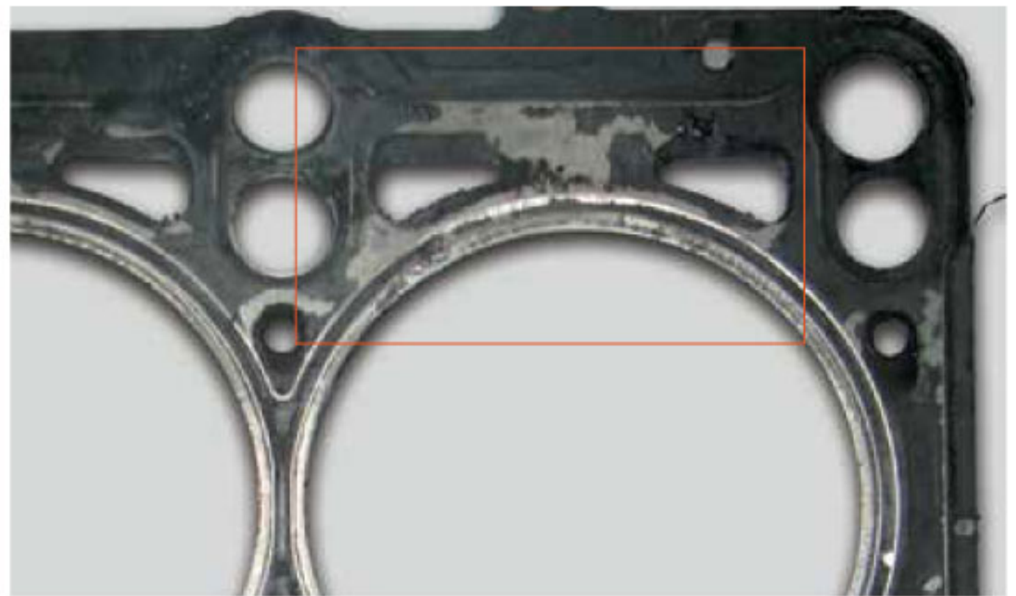
▲ Elastomer coating damaged by overheating
