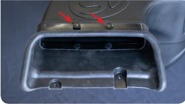
**20** Remove the MAF sensor retaining screws and the MAF sensor from the stock air box lid.
