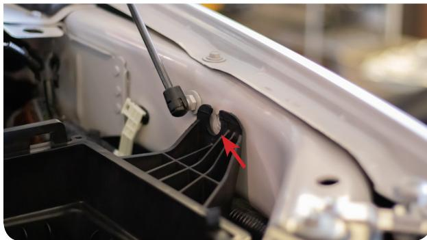
**9** Disconnect any harness clips attached to the stock air box.
