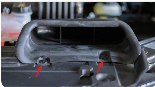
**11** Lift and remove the stock air box from the vehicle.
