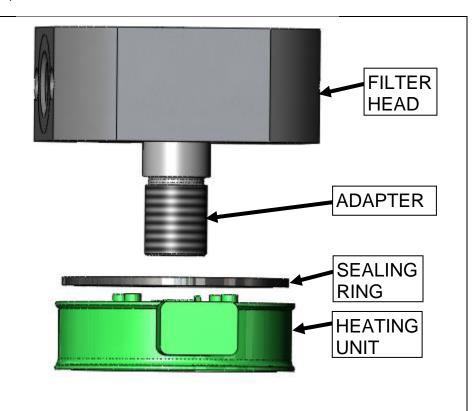
b) Place a dab of blue thread lock onto the adapter then, thread the supplied panel nut (#1500342) onto the threaded stud, thereby securing the heater in place.
