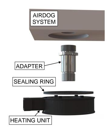
b) Place a dab of blue thread lock onto the adapter then, thread the supplied panel nut (#1500342) onto the threaded stud, thereby securing the heater in place.
