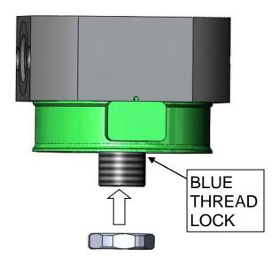
IMPORTANT: Clean excess thread locker from the exposed threads before installing filter otherwise the filter may be difficult to remove at the next service interval.
