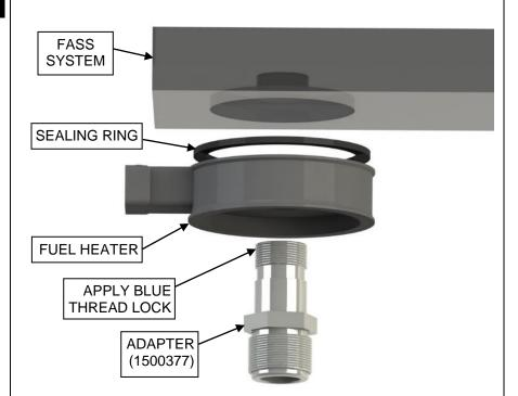
IMPORTANT: Clean excess thread locker from the exposed threads before installing filter otherwise the filter may be difficult to remove at the next service interval.
