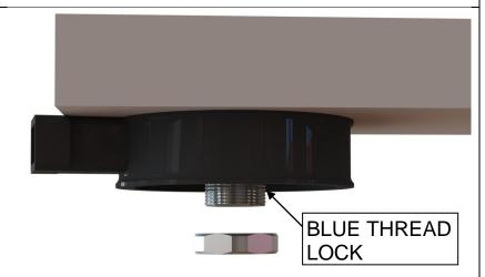
IMPORTANT: Clean excess thread locker from the exposed threads before installing filter otherwise the filter may be difficult to remove at the next service interval.
