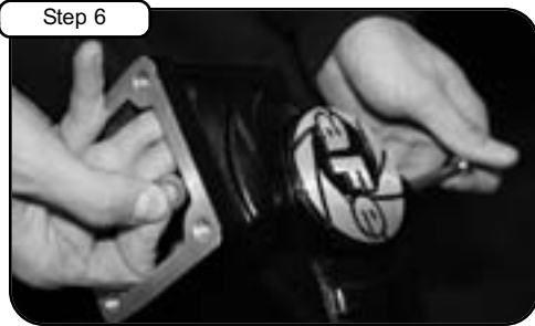
Step 6 Insert the 2 shorter M8 socket cap screws through aFe manifold. Hold washer against inside mounting flange of aFe manifold and feed screw completely through. Insert the two longer M8 screws w/ washers through the outside mounting bosses.
