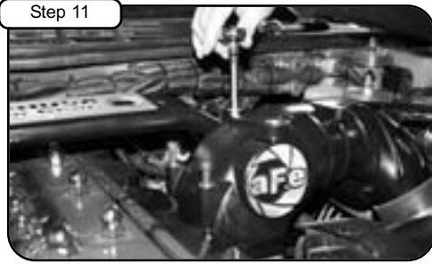
Step 11 With 6mm hexagonal bit provided and 6mm socket, install the four mounting screws. Do not tighten completely!
