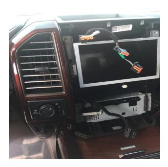
3. Remove the top 2 or 3 buttons from your stock bezel depending which model you have. Remove the 5 orange tabs marked in red in the picture below. Take your T10 bit and remove all screws from the dash bezel.
