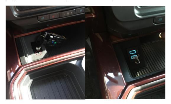
10. Plug all Factory plugs back into your dash bezel and install back on the dash. Install the (2) 7mm bolts up top and clip in the top pocket. Now you have completed your Retro Customz iPad In Dash install. Enjoy!
