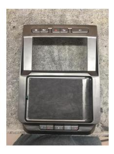
8. Flip Your Dash Bezel over with the iPad in place and insert your lighting cable. Using a 2 part epoxy or JB quick weld you're going to secure your charge cable to your bezel. During this process keep the iPad in the bezel so the charge cable is aligned perfect. Be careful not to let the epoxy run through onto your iPad. Let epoxy fully cure before you remove your iPad. Once cured you're ready to install your dash bezel into your truck.
