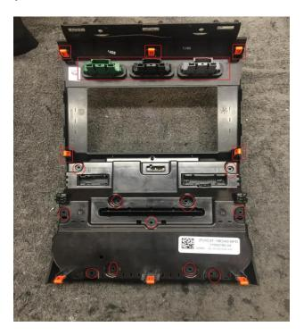
4. Remove back cover, circuit boards, bottom controls and take your top buttons and 6 of the shorter T10 Screws and put them aside as all of these things will be mounted to your new iPad dash bezel.
