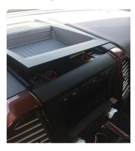
2. Once 7mm bolts are removed pull the dash bezel towards you and it will come loose. Unplug the necessary connections so the bezel can be removed from the truck.
