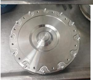
Once fully assembled, the end play of the torque converter should be verified, to ensure the stator spacing is correct. This can done by lifting the turbine using a end play tool, and measuring the play with a dial indicator or by using and end play gauge stand.
