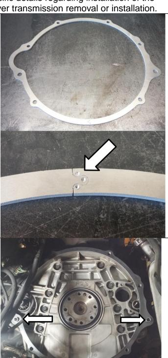
Remove the factory dowel pins and install the supplied longer pins.
