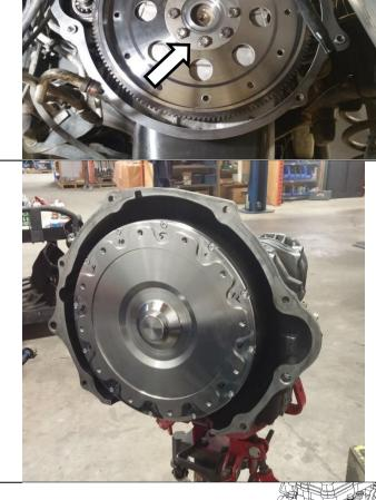
Install the transmission back into the truck.
