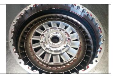
Assemble the turbine and piston into the impeller and install the clutch pack as outlined in the Clutch Service section of this manual.
