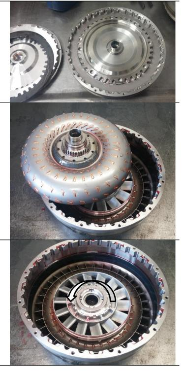
Check the stator and bearings for wear or damage. Ensure the sprag only turns freely in one direction (counter-clockwise when viewed as shown, from the turbine side of the stator).
