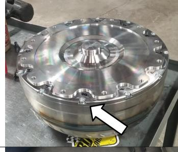
Remove cover plate from the torque converter. This may require a rubber mallet to tap around the outside to break it free.
