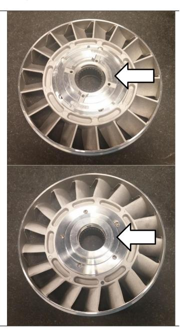
The easiest way to measure the thickness is to lay the stator on some blocks and use a height gauge.
