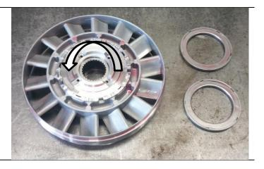
If stator is found to be ok, skip to reassembly of the converter. If replacing the stator with a different unit, continue with the steps below.
