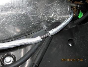
23. Find a place to secure the remote reservoir for the new hydraulic assembly. I attached mine utilizing a spot on the top part of the fire wall just below the hood. I did have to remove the driver's side battery to get my drill in there to install the self tapping screws. Put it where ever you want, just be sure it's not in the way of anything and isn't going to be damaged.
