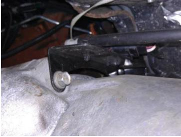
**NOTE:** There is not enough clearance between the exhaust hanger on the downpipe and the transmission bell housing for you to slide the transmission back. You will need somebody to pry between the transmission and the hanger while you wiggle the transmission back to get enough clearance. If you don't want to do this, you must remove the downpipe.
