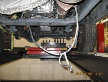
8. Remove the clutch slave cylinder from the driver's side of the bell housing by removing the two nuts holding it on, it will slide out in your hand. Loop it over to the driver's side frame rail and set it out of the way. The front driveshaft makes a nice shelf for this.
