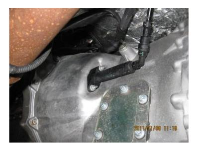
9. Support the transmission with a good transmission jack and securely strap it down. It will try to rotate with the transfer case hanging off of the side and if the jack isn't centered it may try to slide forward or back.
