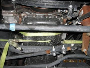
11. Remove the two bolts on the passenger side bottom corner of the bell housing that attach the exhaust mount to the transmission. You can apply some force to this and rotate it counter clockwise so you can slide it off of the hanger rod on the downpipe. Then remove the other six bell housing bolts. The top two bolts on the driver's side are holding a bracket assembly that's used to support a wiring harness and vent hose. It's easy to remove, just be aware of it.
