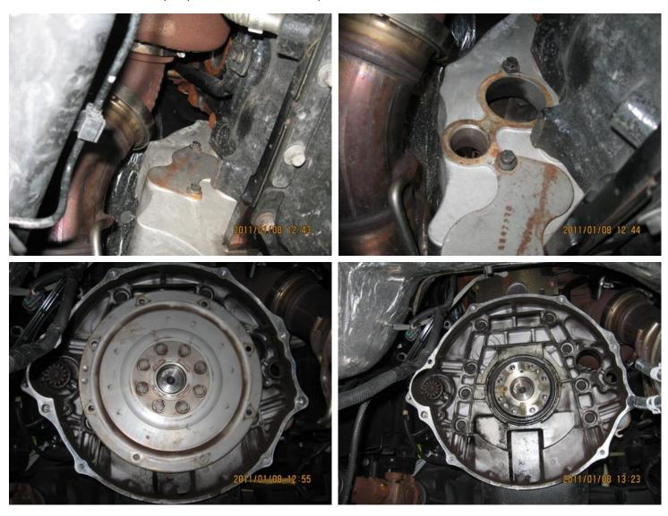
15. Remove the clutch fork assembly and the throw out bearing from the transmission bell housing. It is sitting on a pivot ball on the passenger side and will pop out with very little pressure.
