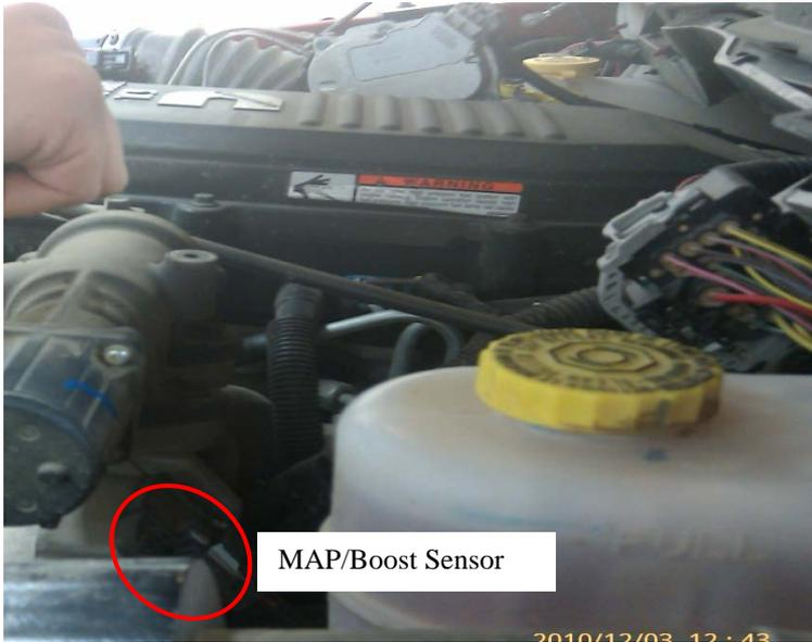
6) Unplug the MAP sensor and Plug in the Female plug from the module into the sensor
