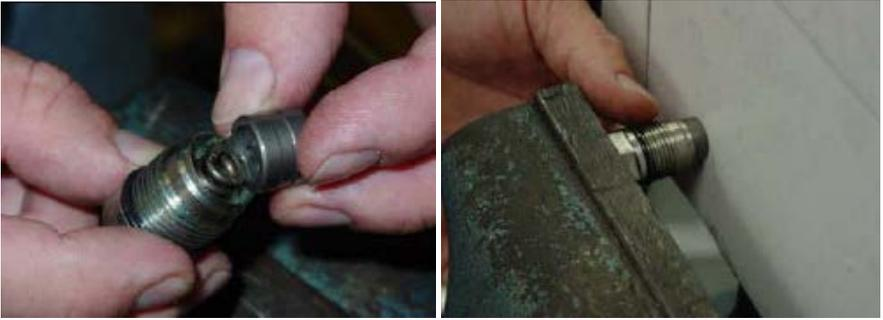
9) Making sure you don't lose any parts, replace spring into relief valve and put tip back together.
