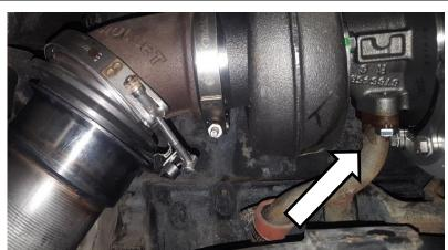
11.Install the oil supply line (reuse OE line).
