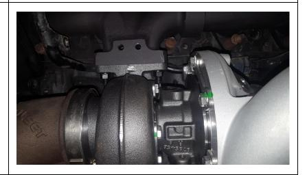
9. Install the supplied (1453152) oil supply fitting onto the turbocharger.
