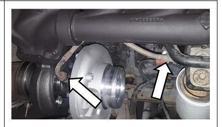
12. Connect the CAC pipe and boot to the turbo charger. Tighten clamps.
