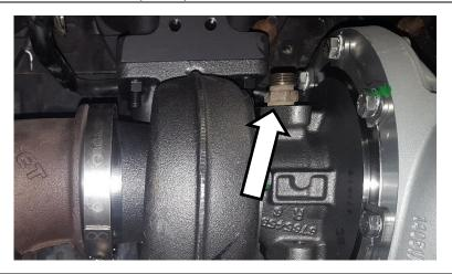
10.Install the supplied corrugated oil drain (Not shown in picture).
