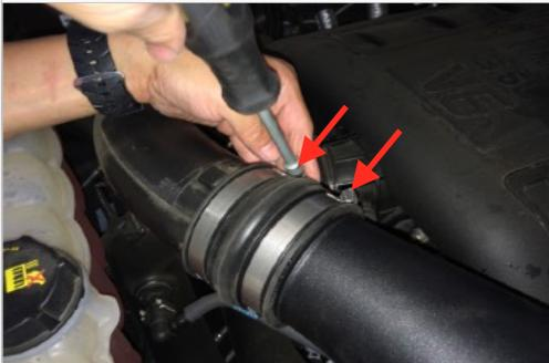
31. Tighten both #72 Hose Clamps (T) on the driver side.
