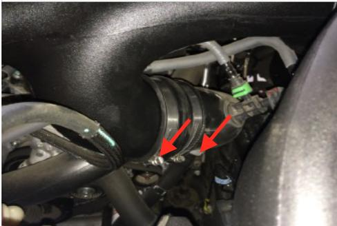
32a. For 2015-2016 Models and 2017 2.7L EcoBoost Only. Reconnect the wiring harness back into the IAT sensor.
