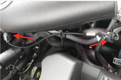
33a. For 2015-2016 Models and 2017 2.7L EcoBoost Only. Insert the two wire harness clips disconnected in Step 11 into the holes on the side of the Air Box (A). For 2017 3.5L EcoBoost Only. Insert one wire harness clip into the hole under the S&B Logo and use zip ties secure the other wire harness clip away from any hot surfaces and moving components that may cause damage.
