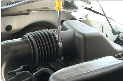
**3.** Loosen the hose clamp at the tube leading to the turbo inlet on the passenger side.
