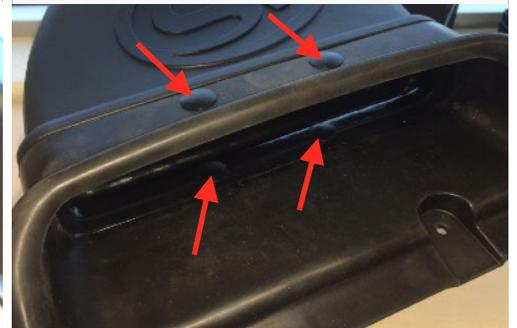
18. Install the Grommet (V) into the Intake Tube (B).
