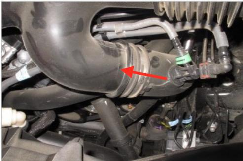
**5.** Unhook the two latches on the stock air box. **For 2017 3.5L EcoBoost Only.** Disconnect the clip securing the vacuum line on the stock air box.
