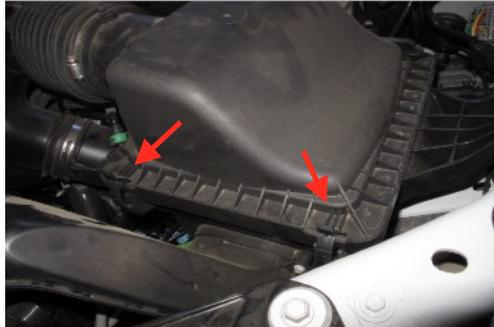
**6.** Lift and remove both the lid and stock air filter.
