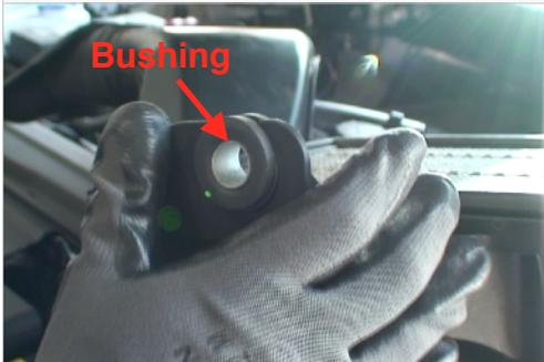
14. Install the grommet into Air Box (A) first and then install the metal bushing from the inside.
