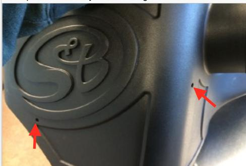
33b. For 2017 3.5L EcoBoost Only. Reconnect the clip securing the vacuum line into the slot on the Vacuum Line Bracket (W).
