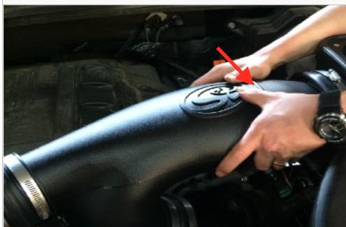
**26.** Once the bead is up to the Cuff (C). Slide the Air Filter (D) onto the Intake Tube (B).
