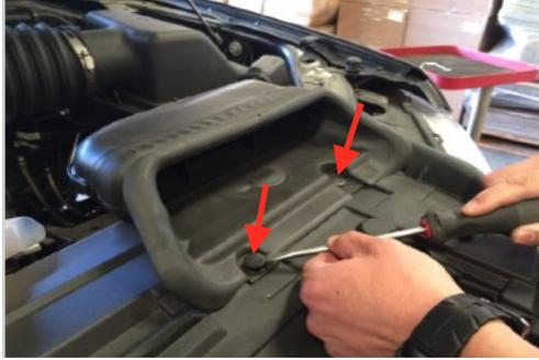
11. Disconnect the two wire harness clips on the stock air box.
