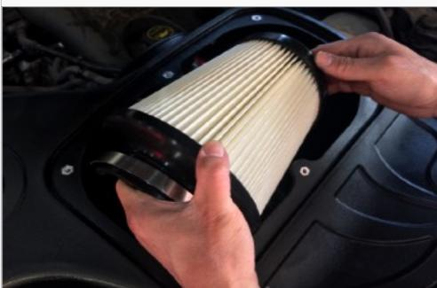
**25.** Feed the Intake Tube (B) through the Cuff (C) and into the air box until the air filter fits up to the bead. As you are feeding, try to align the air intake tube with the turbo inlet tubes..
