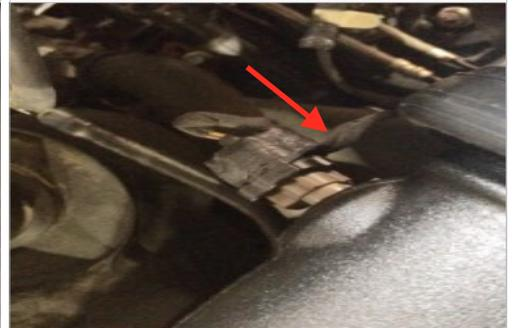
32b. For 2017 3.5L EcoBoost Only. Connect one end of the IAT Sensor Extension Harness (AA) into the stock IAT harness and the other end into the IAT sensor. Use zip ties to secure the extension harness from any hot surfaces and moving components that may cause damage.
