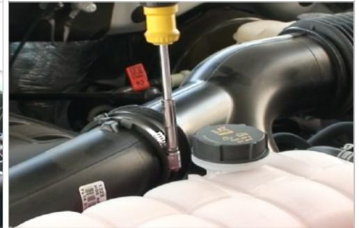
**4.** Loosen the hose clamp at the tube leading the turbo inlet on the driver side.
