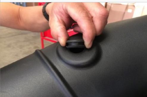
19. Install the Hump Coupler (P) with Hose Clamp #52 (R) into the Intake Tube (B) that leads to the passenger side. Do not tighten the hose clamps. Install the Straight Coupler (U) and Hose Clamp #72 (T) that leads to the driver side. Do not tighten the hose clamps. To make the installation onto the turbo inlet tubes easier, try to slide the coupler in over the air intake tube as much as possible.
