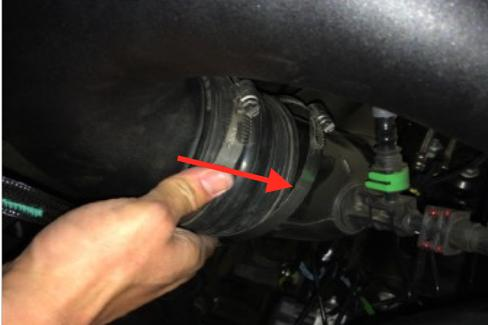
29. Slide the Hump Coupler (P) over the passenger side turbo inlet tube.
