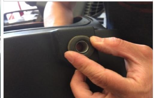
15. **For 2017 3.5L EcoBoost Only.** Install the Vacuum Line Bracket (W) with the 1/4-20 Screw (X), Washer (Y) and Locknut (Z).
